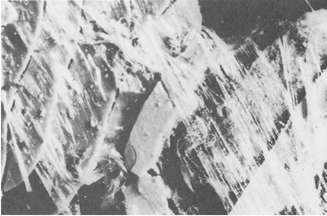
FIG. 2—Photomicrograph ( \times 26 ) of the plastic film spread on the paint surface. In less violent and grazing collisions where softening of the plastic takes place, thin plastic films as seen in this figure are deposited on the vehicle surface. In more violent collisions resulting in plastic melt, the above structure in molten condition is embedded on the vehicle surface giving the characteristic appearance of the marks seen in Fig. 1.
